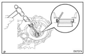
(c) Using SST and a hammer, tap in a new oil seal. SST 09226–10010
